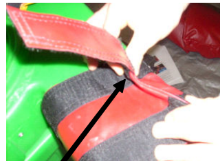
Take out the slack by pinching up the vinyl.
