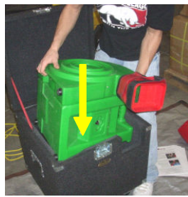
Put blower ON ITS SIDE and lower into the sound case.
