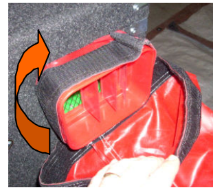
Pinch the extension piece and attach the air tube around the nozzle.
